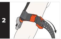
Insert the tip of the strap through the opening in the buckle. Grip the strap close to the buckle and pull hard and steady against the buckle until it stops. Maintaining tension, press the strap back upon itself to hold it in place.
